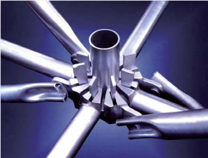
8 holes in one ring: Big hole: for Diagonal, Level Diagonal Small hole: for Horizontal
